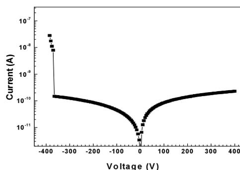
**Fig. 1** The leakage current variation of the detector with applied voltage.
