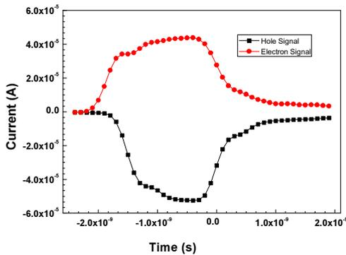
**Fig. 3** Transient current response of diamond detector for electrons and holes due to an alpha particle.
