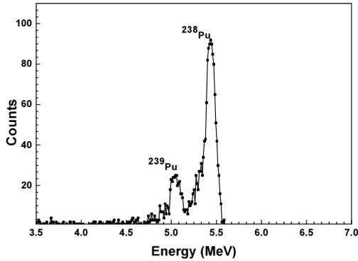
**Fig. 2** Alpha spectrum of detector obtained using dual alpha source of  $^{238}\text{Pu}$ (5.156 MeV) and  $^{239}\text{Pu}$  (5.499 MeV).
