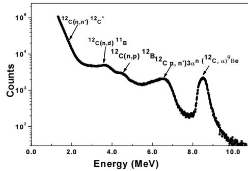
**Fig. 4** Pulse height spectrum with diamond detector for fast neutrons showing various peaks for possible nuclear reactions between neutron and carbon.
