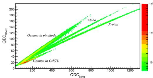
FIG. 1: PID curve showing  $\alpha$ , proton and gamma observed in the experiment.
