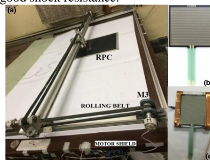
Fig. 1: Photographs of (a) the 2\text{m} \times 2\text{m} AASS, (b) Force Sensitive Resistor (FSR) sensor and (c) Jig equipped with FSR sensor.
