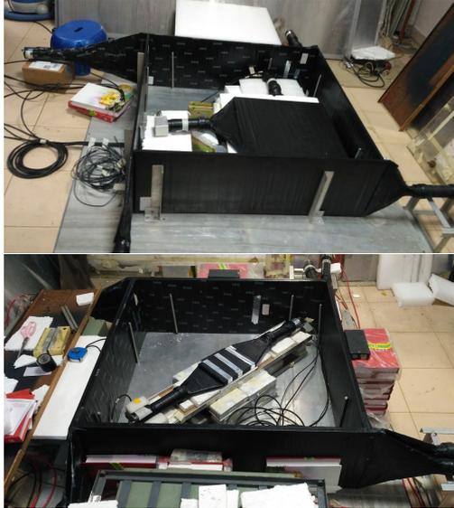
FIG. 1: Photographs of the MuL (top) and MuS (bottom) trigger detectors inside the CMV detector with the top layers removed.
