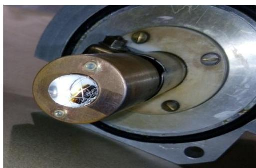
Fig. 1: Assembly of plastic scintillator and Si-PM inside copper tube
