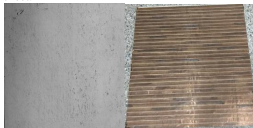
Fig. 1 (a) Silicon Fiber Sheet (SFS) of 1m × 0.5m (b) pickup panels of size 1m × 1m of SFS based.
