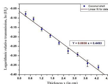
FIG. 3: Logarithmic relative transmission plotted against thickness of coconut samples.
