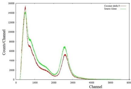
FIG. 1: Spectrum of 662 keV gamma rays obtained with and without coconut shell as an absorber.
