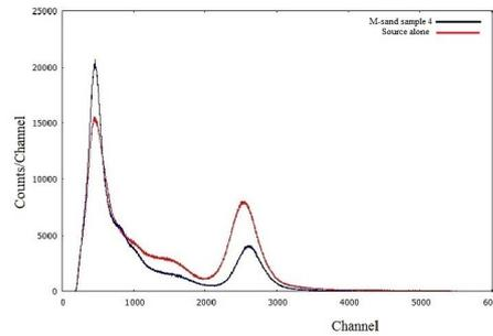
FIG. 2: Spectrum of 662 keV gamma rays obtained from concrete 4(msand sample) reinforced with coconut shell.
