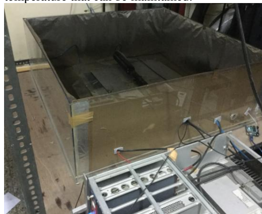
Fig. 1: Box Photograph of controlled environment box of acrylic sheet.
