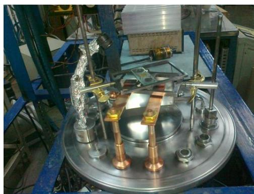
**Fig. 1** Setup used for the evaporation of  $^{130}\text{Te}$  in High Vacuum Evaporator chamber at IUAC, New Delhi.
