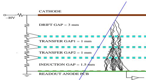
FIG. 1: A schematic of a triple GEM detector.
