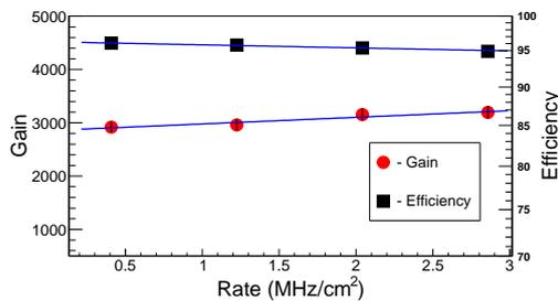
FIG. 2: Variation of the efficiency and gain of the detector with the rate of incoming particle.
