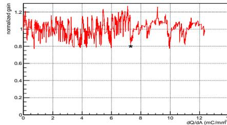
FIG. 3: The Variation of the normalised gain with accumulated charge.
