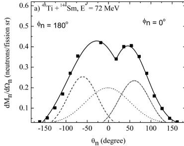
FIG. 2: Experimental neutron angular distribution (solid square) along with the angular distribution obtained from multiple-source fitting (solid line). The angular distribution of different sources; CN (dotted line), fragment1 (dashed line), fragment2 (dashed dotted line) for  $^{48}\text{Ti}+^{144}\text{Sm}$  system at 72 MeV of excitation energy for different  $\phi_n$  corresponding to symmetric mass cut.
