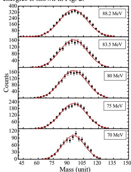
**Fig. 2** The mass distributions of fission fragments for the system  $^{12}\text{C} + ^{178}\text{Hf}$  at different lab energies. The Continuous line represents the Gauss fit to the experimental data.
