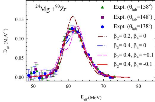
FIG. 1: Quasi-elastic barrier distribution determined from QEL excitation functions measured at three backward angles. Different lines correspond to CCQEL calculations for different values
