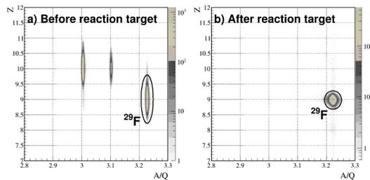
FIG. 1: a) Particle identification spectrum before the reaction target at focal plane F8 of BigRIPS. b) Particle identification spectrum after the reaction target at the final focus F11 of the ZDS. This spectrum is obtained with the gate on  $^{29}\text{F}$  before the reaction target. Particle identification was performed using  $B\rho$ -ToF- $\Delta E$  measurement.
