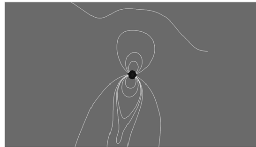
FIG. 1: Earth's magnetic field line distribution used in the simulation.
