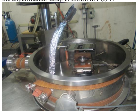
Fig. 1: Experimental setup for the deposition of the tungsten isotopes 182 W, 184 W, and 186 W.
