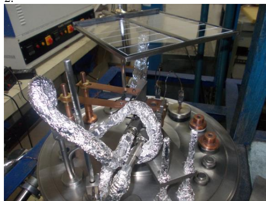
Fig. 2: Experimental setup for the preparation of the carbon backing.
