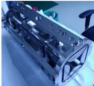
Fig.2. The QT with the poles mounted at different locations. The outer SS jacket is not shown.
