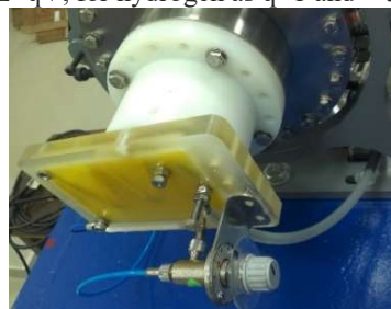
Fig.1. The ion source assembly with the needle valve for the controlled gas flow.
