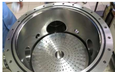
Fig.4. The Scattering chamber with all the rotary and liner drive. The holes are to set the detector in any desired positions.
