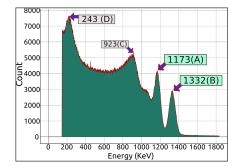
FIG. 2: a)  $^{60}Cobalt$  gamma spectrum calibrated using the known photopeaks labelled A & B. The compton edge corresponding to 1173keV photopeak and backscatter peak calculated with this calibration are also labelled as C & D respectively.
