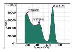
FIG. 3: a) <sup>137</sup>Cesium gamma spectrum showing the photopeak(A), Compton edge(B), and Backscatter Peak(C).
