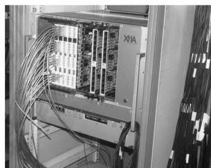
FIG. 1: Digitizer based pulse processing and data acquisition system of UGC-DAE CSR, Kolkata Centre being used at the INGA setup in VECC.
