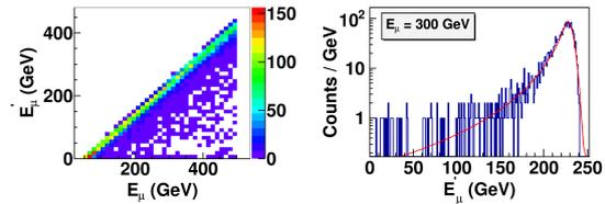
FIG. 2: 2D histogram showing  $E'_\mu$  vs  $E_\mu$  (left) and  $E'_\mu$  distribution 300 GeV (right) incident muon energy fitted to Crystal Ball fit function (right).
