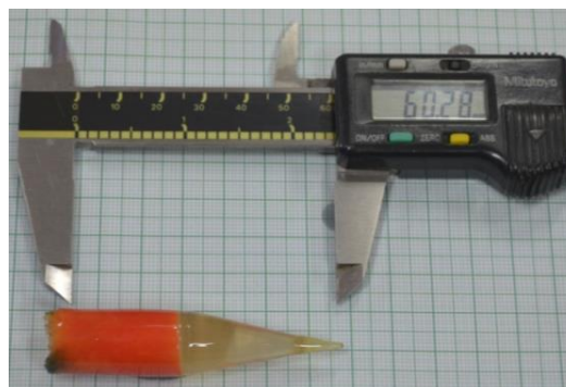
Figure 1. LiI(Tl) single crystal grown via Bridgeman technique.
