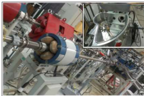
Fig.1 The newly developed neutron beam line at Tandem accelerator (TTT-3) at University of Naples Federico II. The quadrupole can be seen clearly. (Inset) A specially designed chamber for D(d,n)^3\text{He} reaction where the n can be produced.
