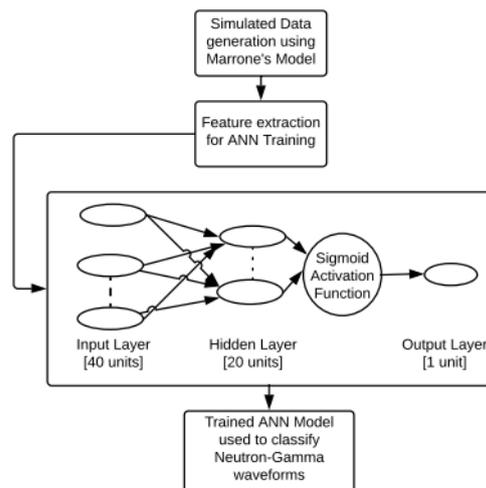
FIG. 1: Workflow used for Discrimination of Neutron-Gamma waveforms using ANN.
