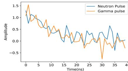
FIG. 3: Intertwining of Neutron-Gamma Pulse input features at elevated noise levels. [ $\mu=0, \sigma=0.2$ ]
