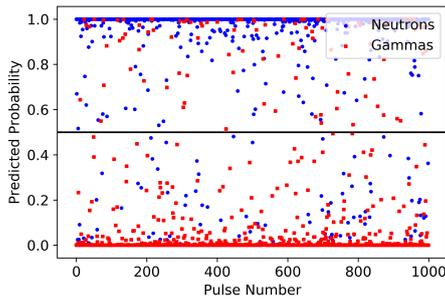
FIG. 2: Prediction of trained ANN model on data with Gaussian noise of  $0 \mu$  and  $0.15 \sigma$ . Classification threshold (black horizontal line) kept at 50%.
