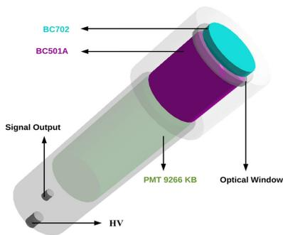
FIG. 1: The simulated schematic diagram of the hybrid neutron detector using GEANT4 [1].
