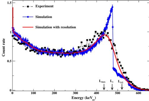
FIG. 3: Light output resolution function of BC501A.  $L_C$ ,  $L_{max}$  and  $L_{1/2}$  correspond to the positions of the Compton edge the maximum probability and the location of halfmaximum intensity, respectively [1].
