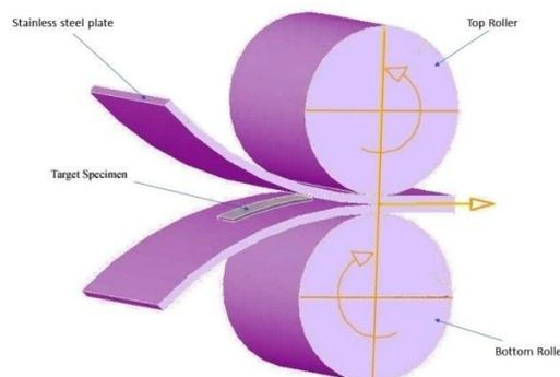
**Fig. 2** Schematic view of rolling machine.
