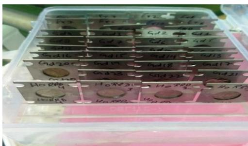
**Fig.3**  $^{156}\text{Gd}$ ,  $^{165}\text{Ho}$  and  $^{166}\text{Er}$  target foils pasted on Al-holders.
