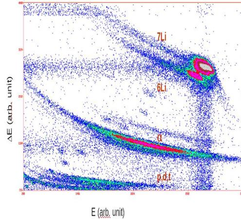
FIG. 1: The Typical 2D spectrum between  $\Delta E$  and  $E$  for one strip of one strip detector telescope. The figure shows clear identification of all the light charged particle up to  $^7\text{Li}$
