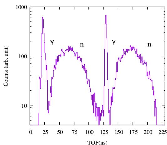
FIG. 2: The neutron time of flight spectrum in  ${}^7\text{Li}$  induced reaction on Tb. The two gamma prompts peaks are corresponding to two beam bunches of the pulsed beam within 213 ns
