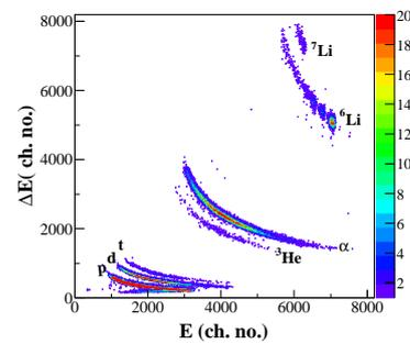
FIG. 1: A typical two-dimensional raw spectrum of one of the vertical strip  $105^\circ$  and  $E_{beam} = 30$  MeV
