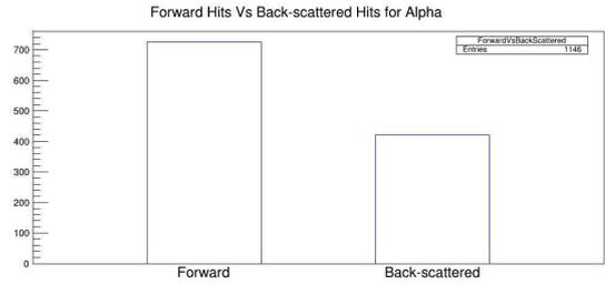
FIG. 4: A study of alphas that are coming from the beam direction vs. those that get backscattered
