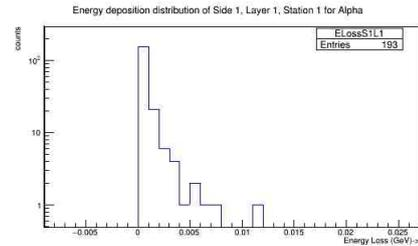
FIG. 5: A study of alphas and how much energy each deposit
