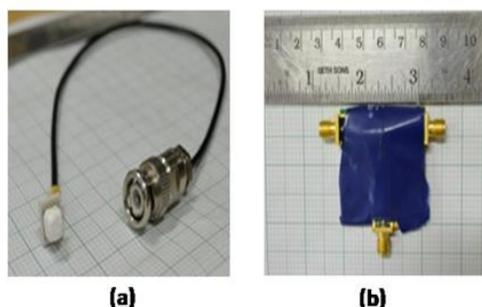
**Figure 1.** GGAG:Ce ( $5 \times 5 \times 5 \text{ mm}^3$ ) crystal coupled with (a) APD (b) SiPM.
