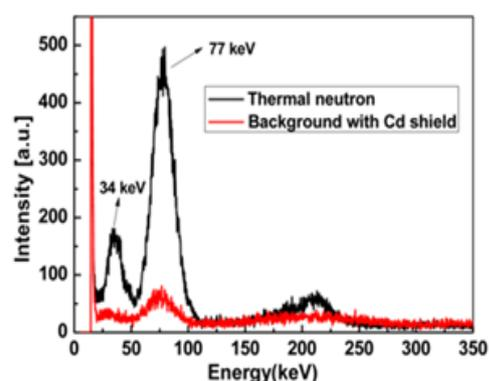
**Figure 2.** The pulse height spectra of thermal neutrons from Am-Be in GGAG:Ce,B scintillator.
