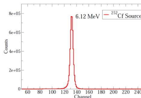
Fig. 1: The alpha spectrum from <sup>252</sup>Cf source.
