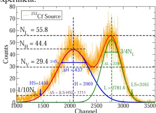
**Fig. 2:** Pulse height spectrum of fission fragments (FF) from  $^{252}\text{Cf}$  with spectrum shape parameters [4, 5].
