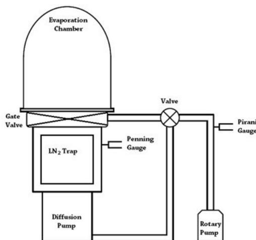
Fig 1. Schematic representation of high vacuum evaporator at IUAC.
