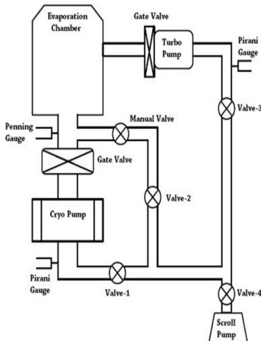
Fig 3. schematic picture of ultra high vacuum evaporator at IUAC used for isotope deposition.
