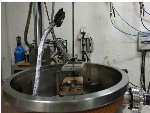
Fig 2. The inside view of ultra high vacuum chamber used for enriched isotope deposition.
