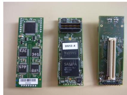
Fig. 1 The FEE R/O chips: the MANAS (left) and Dual SAMPA (middle & right).
