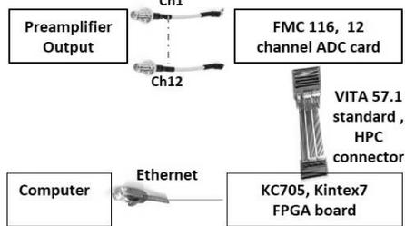
Fig. 1: Electronics block schematic.
