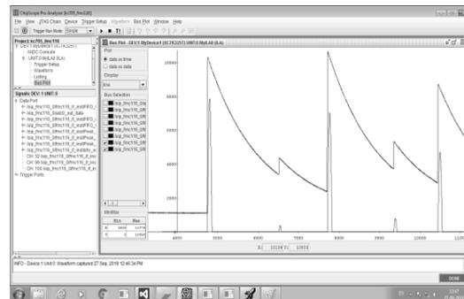
Fig. 2: Digital filter response captured by Chipscope
