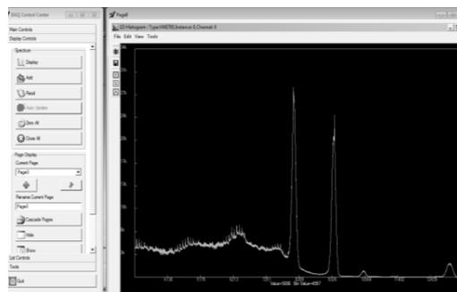
Fig. 4: Co-60 Spectrum from Digital DAQ
