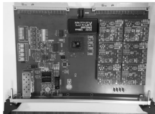
Fig. 3: general purpose VME 6U module
