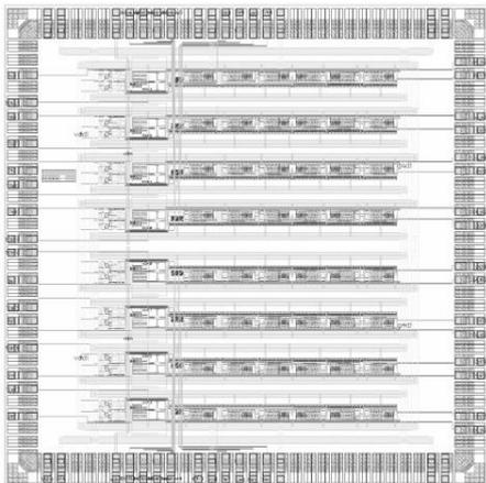
**Figure 3** The layout of the readout ASIC.
