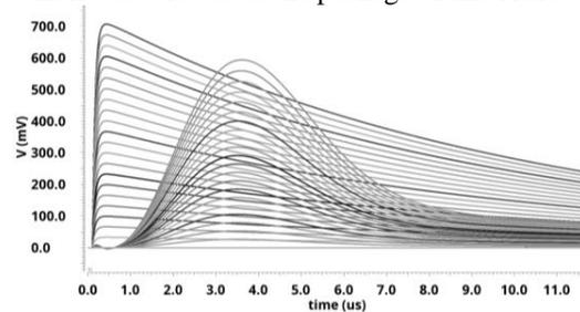
**Figure 4** The typical output of the preamplifier and shaper.
