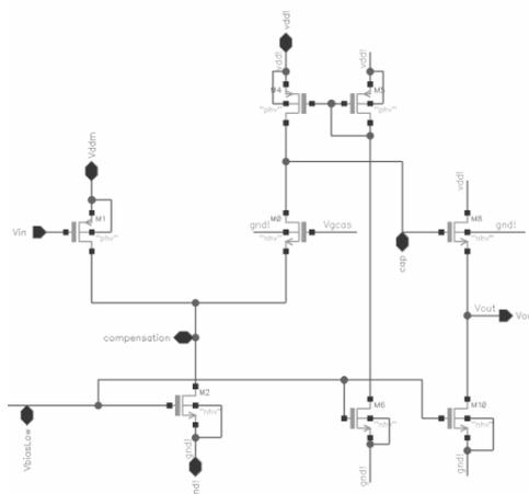
Figure 1 Schematic of Preamplifier Circuit.
