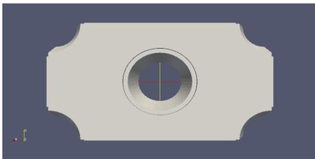
FIG. 1: Unit Cell of GEM detector
