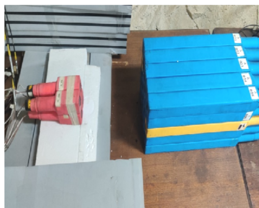
Fig. 1. The experimental setup during the experiment. The LAMBDA array (blue) arranged in 5x5 matrix and the multiplicity filter (red) in 2x2 matrix.
