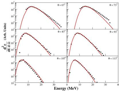
FIG. 2: Alpha particle spectra for  $^{48}\text{Ti} + ^{48}\text{Ti}$  system at 150 MeV. Black circles show the experimental spectra, and red solid line represents CASCADE model calculations with default parameters (refer to text for more information).
