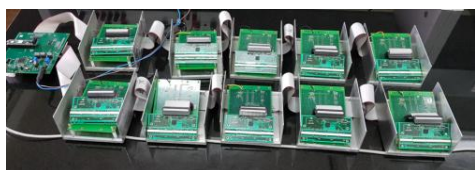
Fig. 2 Detector cards and DAQ electronics for dual energy XBIS.
