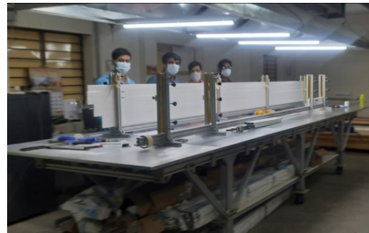
Fig. 4 Assembly of di-counter wall in progress.
