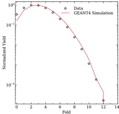
FIG. 2: Comparison of measured prompt gamma fold distribution (open circles) and GEANT4 simulation (red line).
