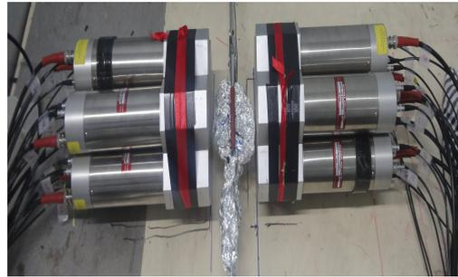
FIG. 1: Photograph of experimental setup consisting of BGO array and fission trigger chamber.
