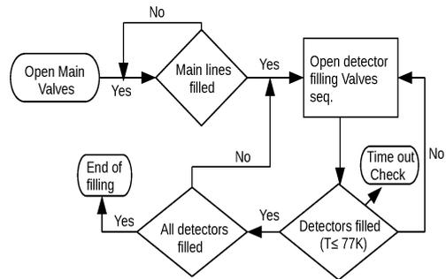
FIG. 1: Algorithm for automatic LN2 filling of detectors
