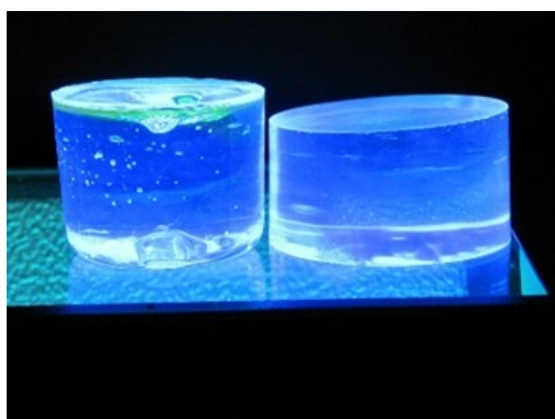
Fig. 1. Photographs of plastic scintillators under UV illumination (left with bubble and right without bubbles)
