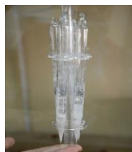
Fig1. Grown CsI:Tl (0.05%, 0.1%, 0.2%, 0.5%) crystal.
