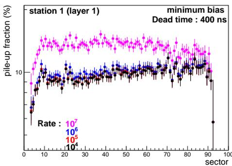
FIG. 2: Pile-up fraction in each sector of the first layer of the first MuCh station for a dead time of 400 ns and for different interaction rates.
