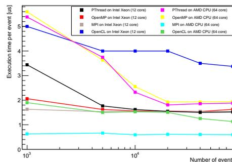
FIG. 1: Execution time per event as a function of the number of events processed at a time for the implementations with pthread, OpenMP, MPI and OpenCL on the Intel and AMD CPUs. The number of threads equals that of the available physical cores (12 for Intel, 64 for AMD).
