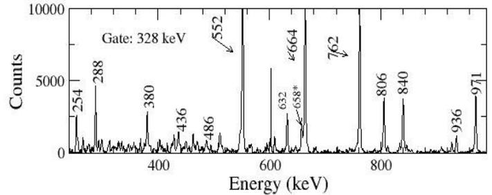
Fig.2: The coincidence energy gate on 328.5keV, showing the decaying transitions of 657.9 keV and ground state band. Several other transition also observed belonging to other bands in  $^{136}\text{Ce}$ .
