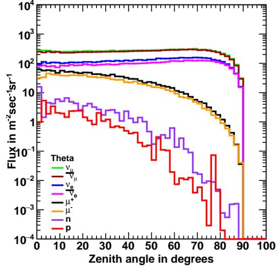
FIG. 2: Flux of the major cosmic ray shower particles reaching at ground level as a function of zenith angle distribution.
