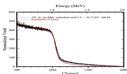
FIG. 3: The RBS spectrum and simulation using XRUMP.
