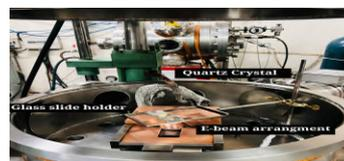
FIG. 2: The high vacuum e-beam set-up at IUAC, New Delhi.
