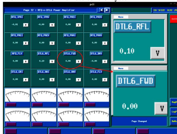
Remote Control of DTL #1 6kW amplifier(RS485 based RF power amplifier)[3]
