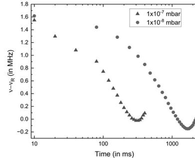
Fig. 2: Variations of the axial frequency of the center of mass with time at  $1 \times 10^{-7}$  mbar and  $1 \times 10^{-8}$  mbar pressure.
